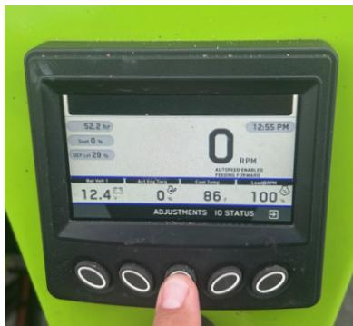
3. Next select the “FEED WHEEL” option by pressing the button to the far-right side. This will bring up the Disengage setting for the Auto-feed. This is the main setting that will be changed in order to feed different diameters of materials.
