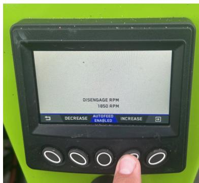
5. To lower the Disengage RPM push the button to the left (Decrease) of the center button. Generally, you will lower the Disengage RPM for smaller brushy materials. This allows the machine to feed the material without the Auto-feed kicking on as often.
