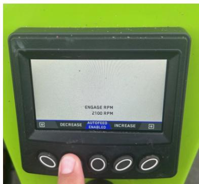
7. By pressing the far-right button while in the Engage RPM screen, you will access the reversing time. This is the length of time that your feed wheel will back the material away from the drum when Auto-feed is activated. You adjust this setting the same as your Engage and Disengage RPM. Use the Decrease and the Increase buttons to adjust the setting up or down. 200 milliseconds is the factory setting for Reversing time.
